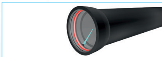
6. Greasing the inner surface of the rubber gasket
