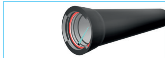
4. Greasing the inner surface of the socket
