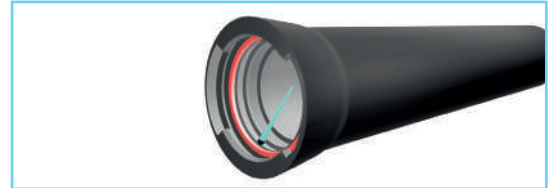
4. Greasing the inner surface of the socket
