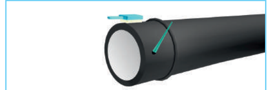
1. Spigot cleaning and greasing
