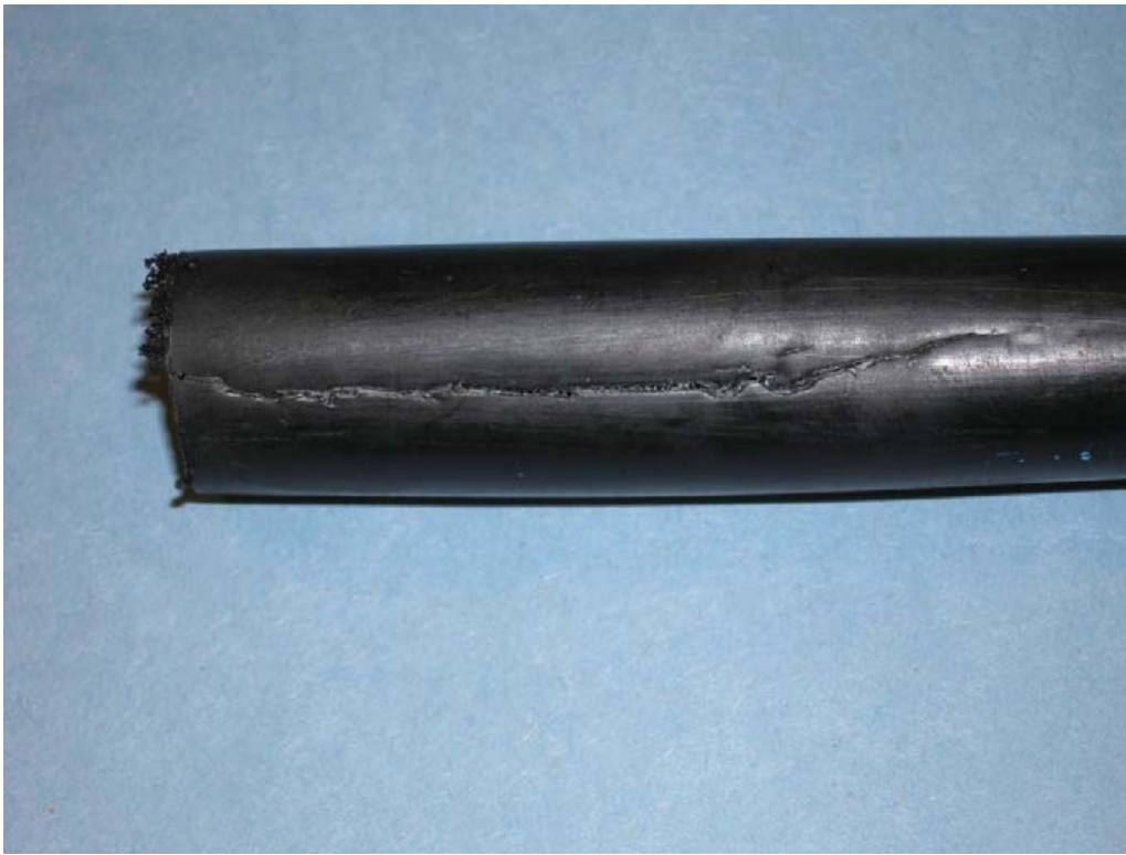
Figure 19. Longitudinal fracture from 5612 Anise CT, Bakersfield, CA .
