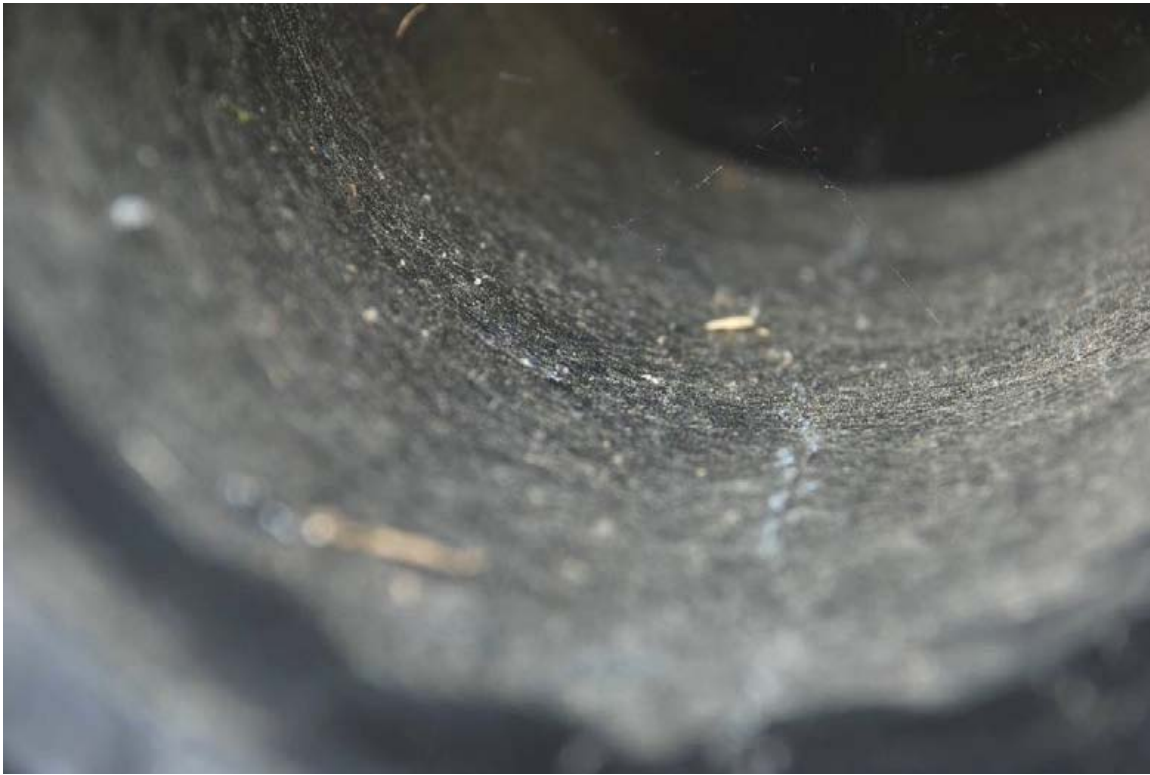
Figure 12. Cracking of Ocoee sample on Pipe I.D.
