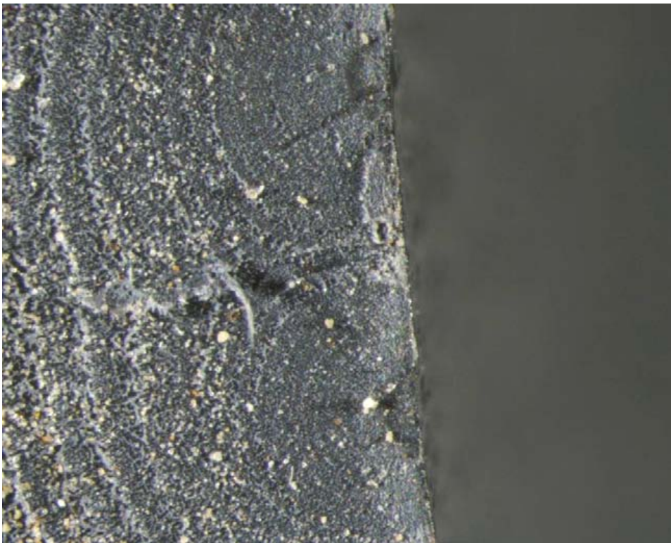
Figure 18. Close-up of fracture origins.
