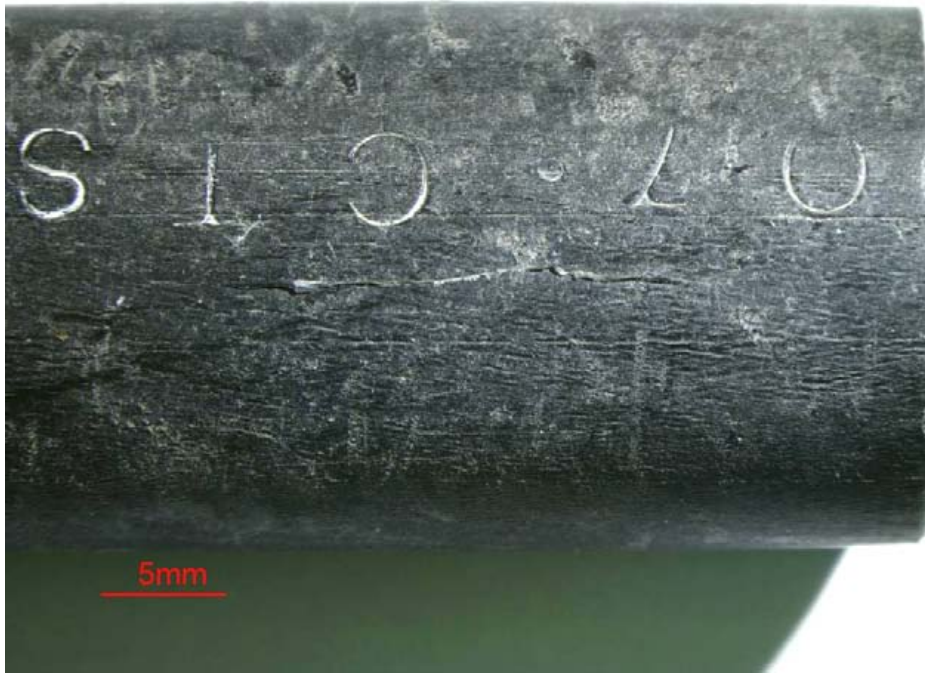
Figure 29. Hamilton, OH sample with longitudinal split.
