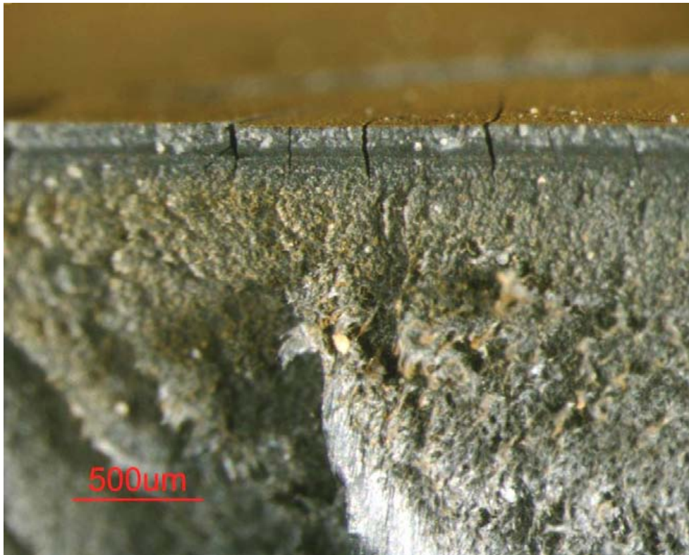
Figure 10. Fracture surface from an adjacent area showing brittle inner surface.
