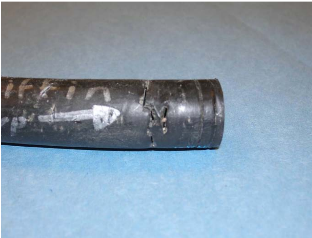
Figure 36. Failure at fitting – Hamilton, OH sample.
