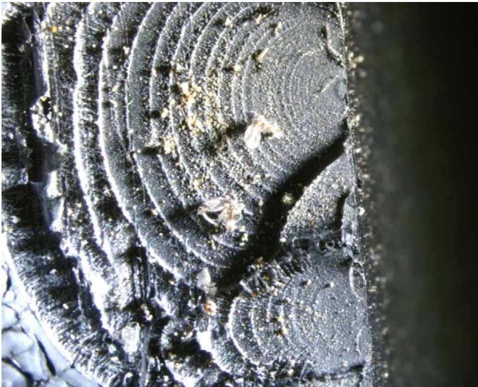
Figure 15. A portion of the fracture surface showing multiple fracture origins and slow crack growth.
