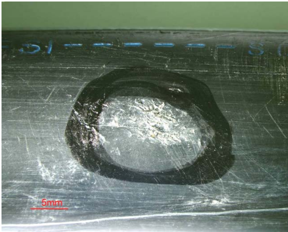
Figure 26. Failure location with outer surface deformation – Bakersfield sample.
