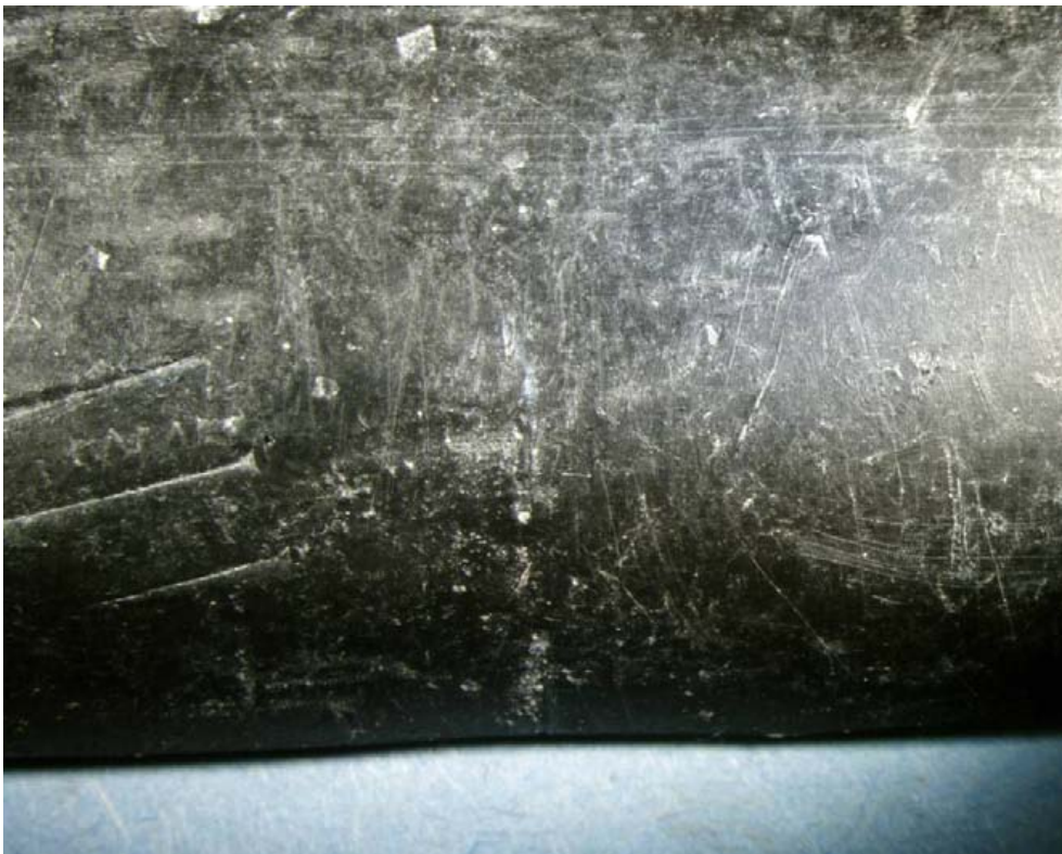
Figure 3. Squeeze-off adjacent to failure location.
