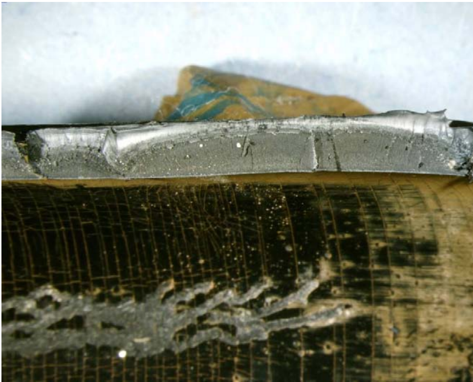
Figure 8. Fracture surface showing multiple initiation sites along the inner surface.
