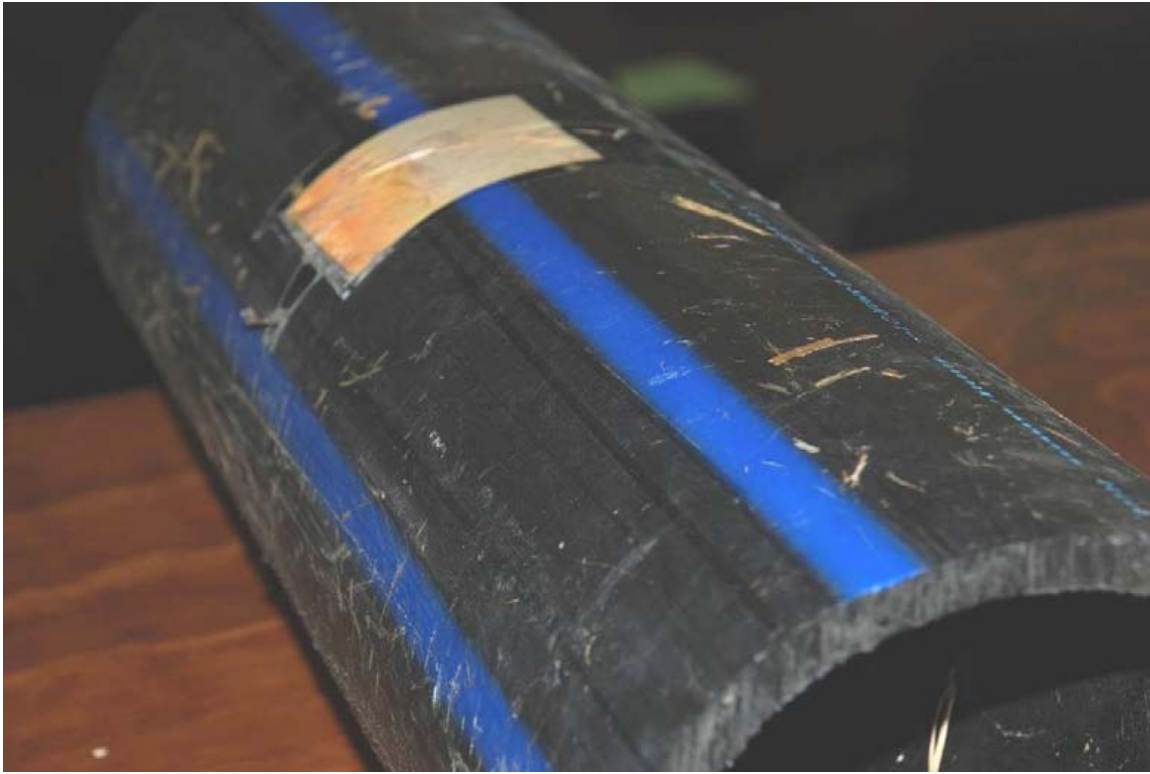
Figure 11. Ocoee 6-inch HDPE pipe sample, as received.
