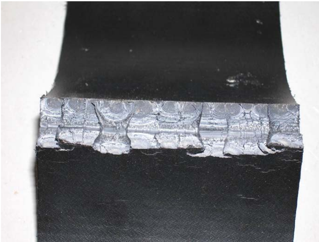
Figure 14. Exposing the fracture surface - Ocoee sample.
