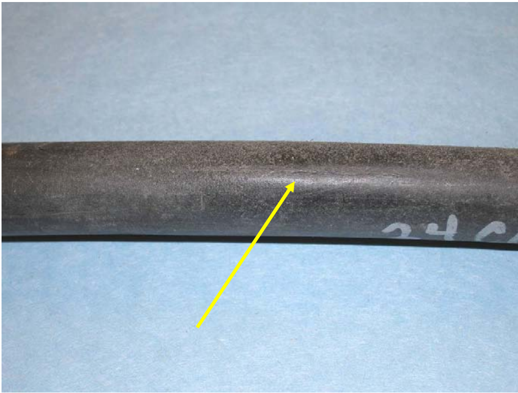
Figure 31. Second Hamilton, OH sample with longitudinal split.
