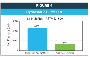
\*Burst pressure at which PVCO pipe failed by ballooning or fracturing.
