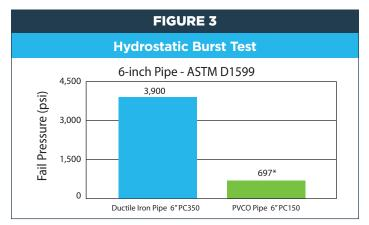
\*Burst pressure at which PVCO pipe failed by ballooning or fracturing.
